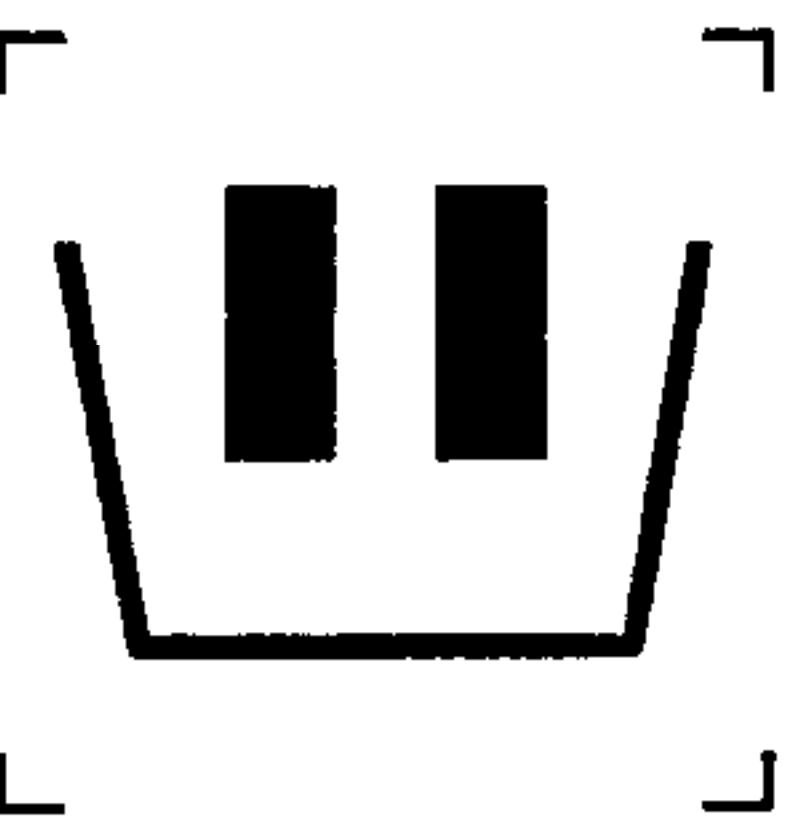
5227 主洗, 纺织品洗衣机 Main wash, textile washing machines
