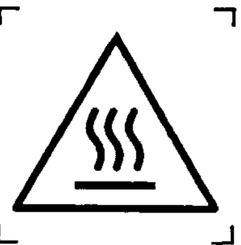
5041 小心, 烫伤 Caution, hot surface
